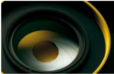
An iris diaphragm with stepless adjustment from f/1.7 to f/4.0 for the optimum matching of brightness to the different cinema projection formats with 12 blades for an almost circular aperture to minimize diffraction.
